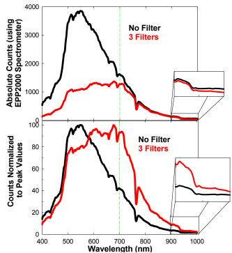
Filters reduce visible spectral response and allow a relative increase in NIR signal.
