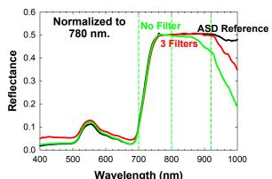
3 layers of filter extend the NIR accuracy of the spectrometer from 800-920 nm.
