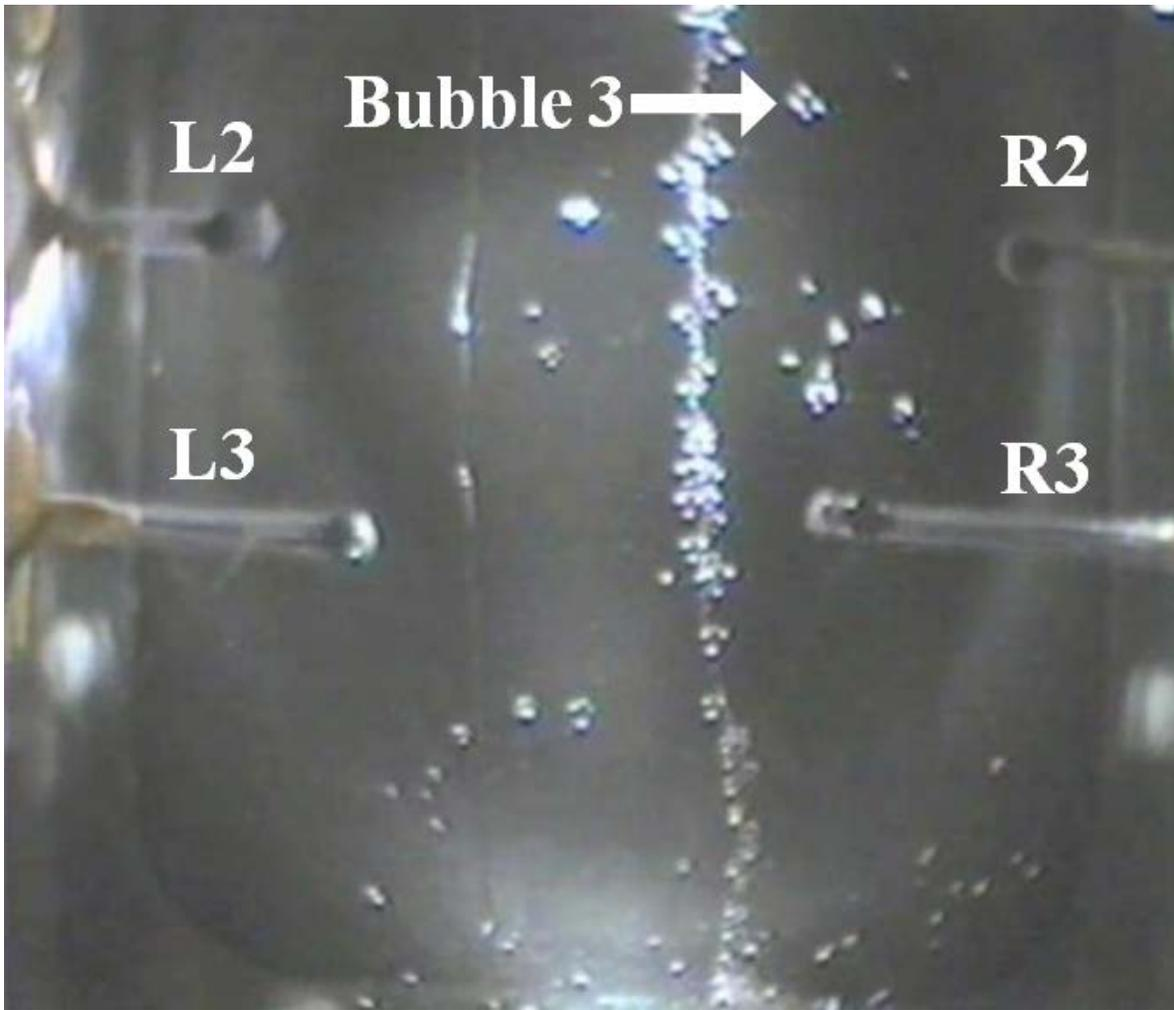
Fig. 9. Photograph of nucleate boiling on a braided wire.
