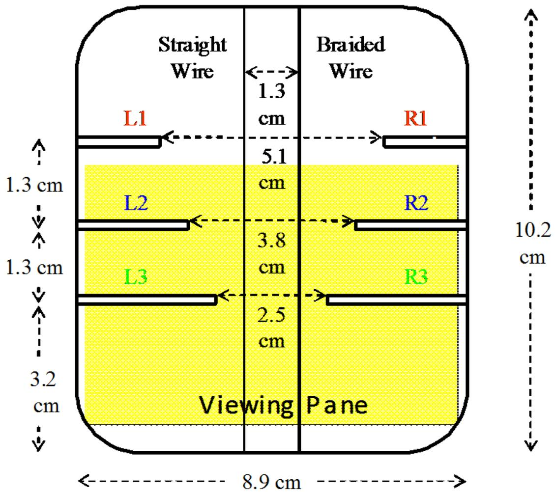
Fig. 2. Chamber cross section schematic.
