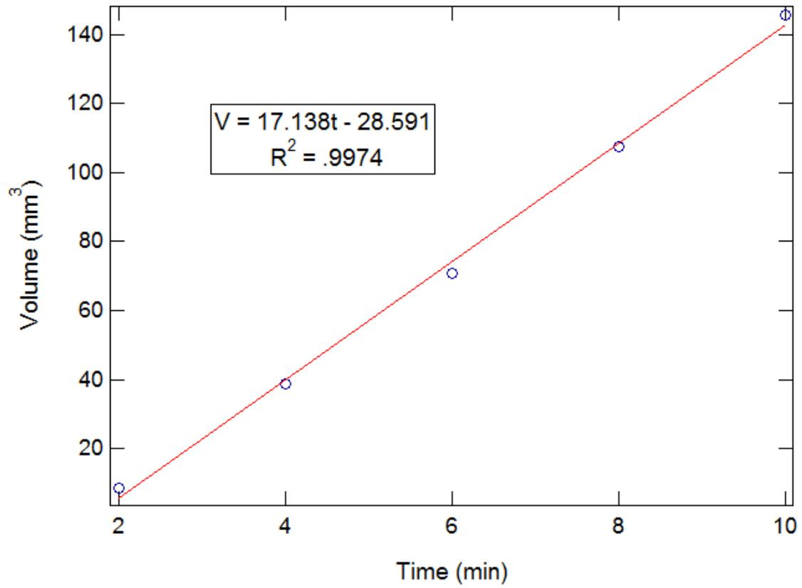
Fig. 6. Total volume of vapor in fluid chamber versus time.
