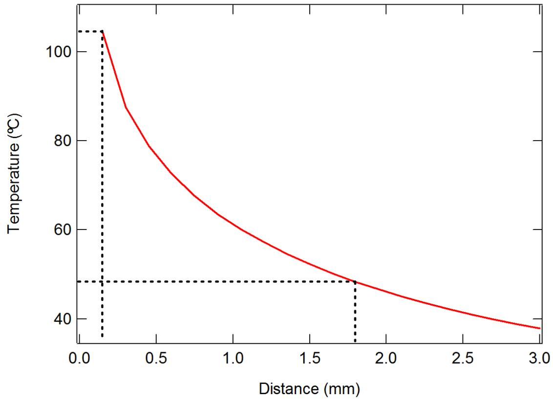
Fig. 4. Temperature of fluid versus distance from center of braided wires from ANSYS modeling.
