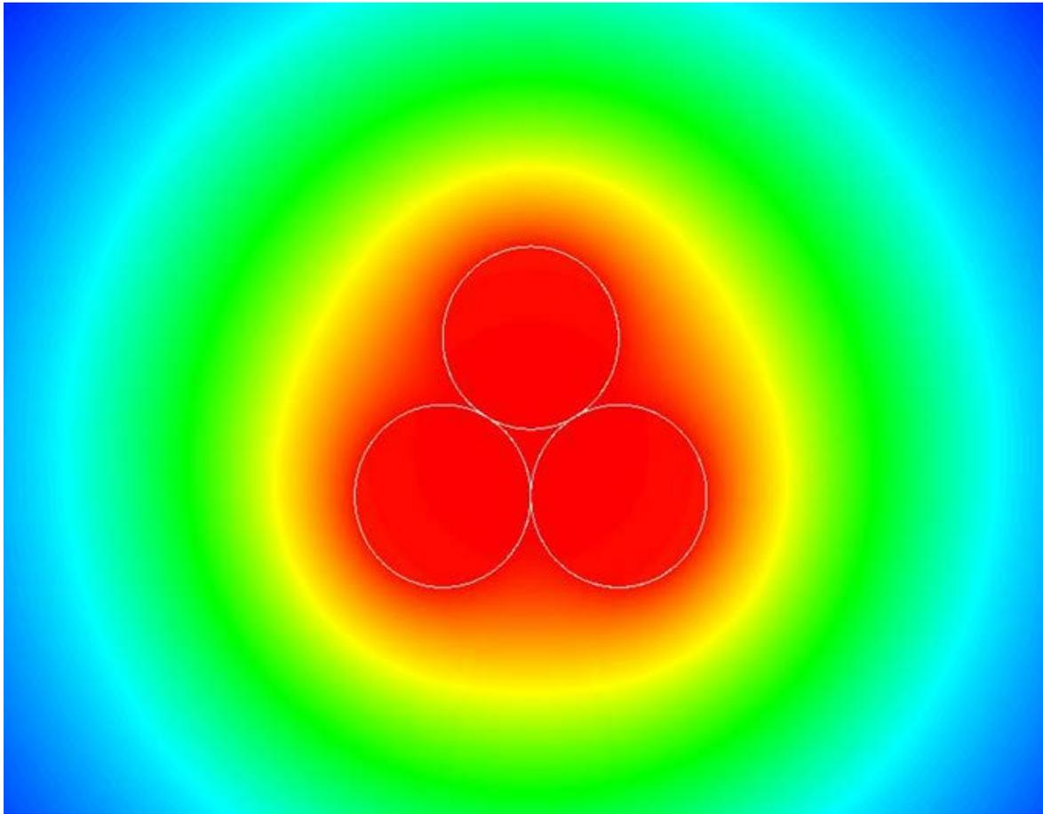
Fig. 8. Temperature contours surrounding the 3 heating wires ( $D = 0.16$  mm) at time  $t = 120$  s.
