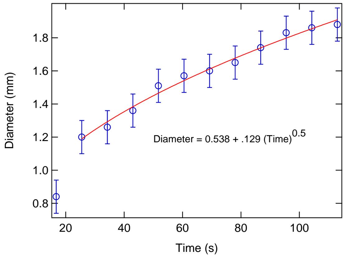
Fig. 5. Measured bubble diameter with respect to time compared to predicted bubble growth.
