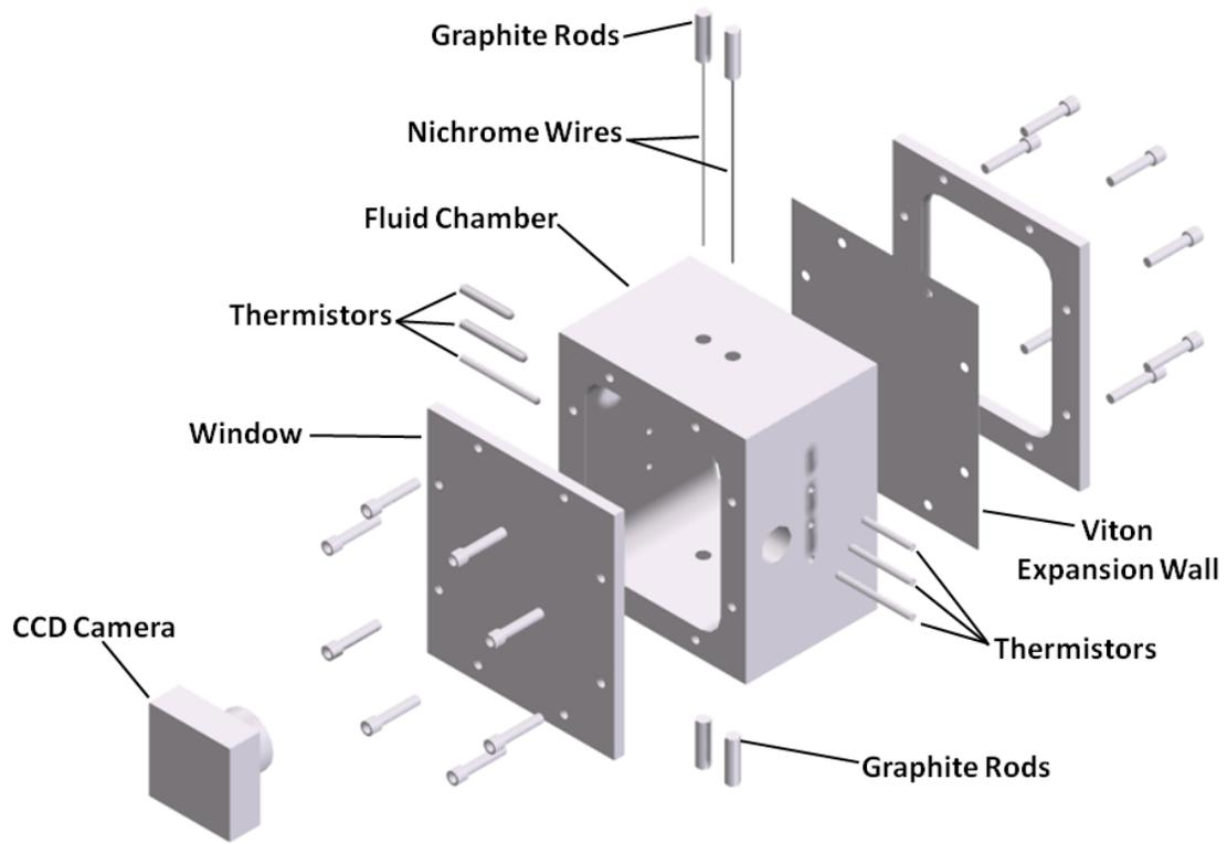
Fig. 1. Diagram of experimental fluid chamber.
