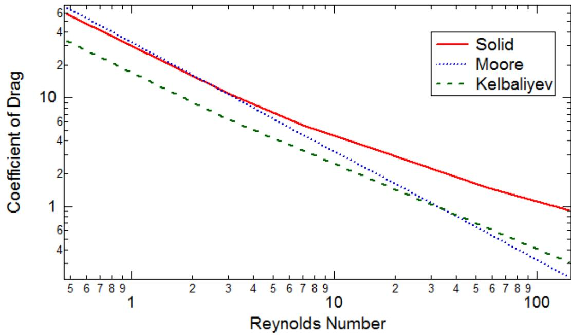
Fig. 10. Comparison of drag coefficient for a solid sphere and a bubble using Moore's and Kelbaliyev's methods.
