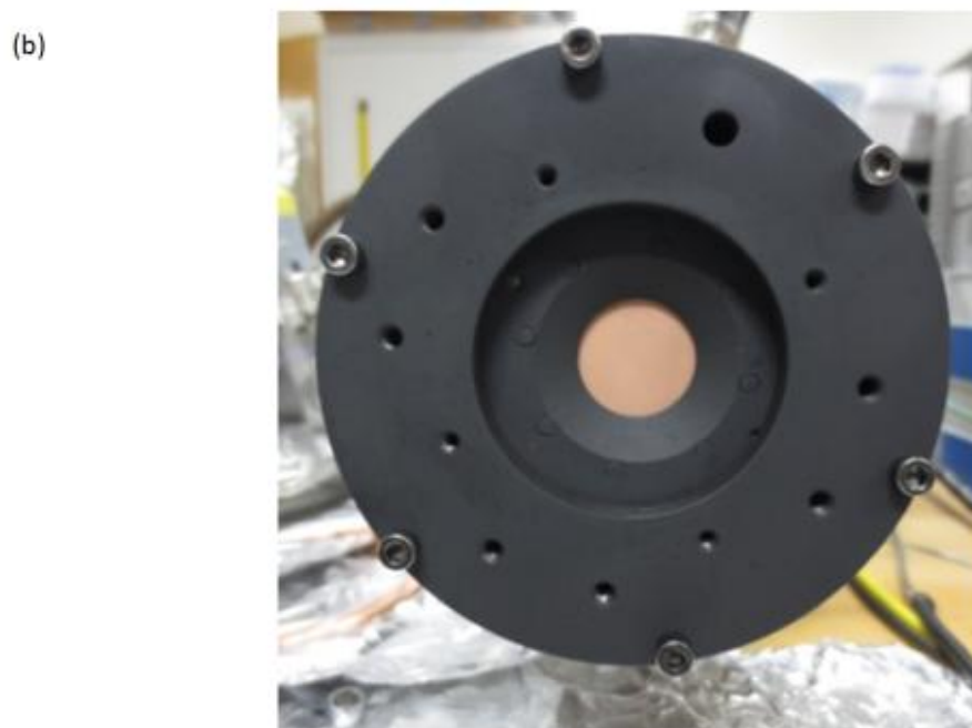
FIG. 3.9. Solid model of sample mounting and image of the Aquadag™ surface. (a) The solid model shows each layer of the mounting assembly for Sample C as called out in the text. (b) The front surface of L was sprayed with a coating of Aquadag™ to reduce reflections.
