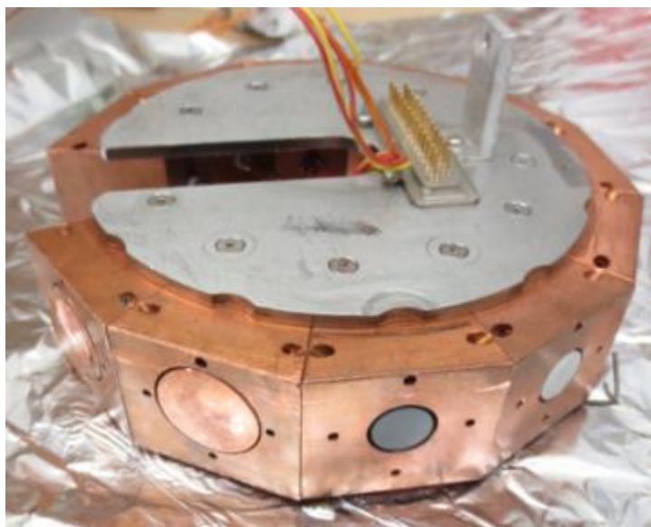
FIG. 3.5. Sample carousel used to house samples for tests A and B.
