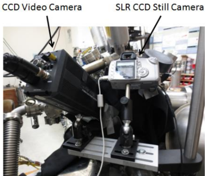
FIG. 3.17. Cameras used for optical detection. CCD video camera (left) and the SLR CCD still camera (right) as they are set up to look at the sample.
