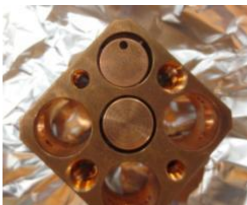
FIG. 3.8. Cu cylinder (top corner) that holds the spring-loaded pin, which makes electrical contact with the back of the sample. This is mounted in the sample round along with the FC (middle), and the other sample slots are left empty.
