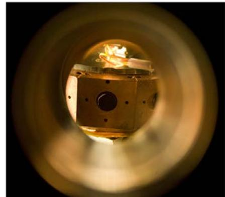
**Figure 1** SLR image looking down port in ultra high vacuum chamber showing sample mounted in carousel.
