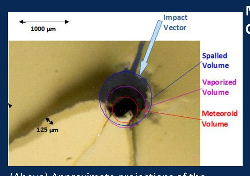
(Above) Approximate projections of the damage due to the micrometeoroid impact.
