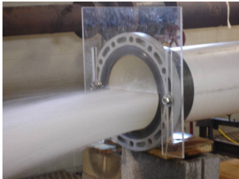
Figure 15. Placement of end cap.
