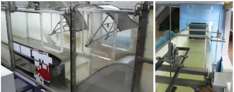
Figure 1 – Physical scale model (left). Upstream flume and point gauge (right)
