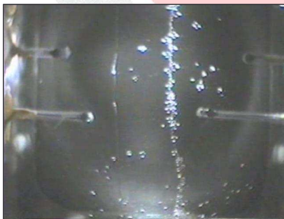
Picture of bubbles growing and departing radially from a braided wire heating element taken from the STS-108 GAS team boiling experiment
