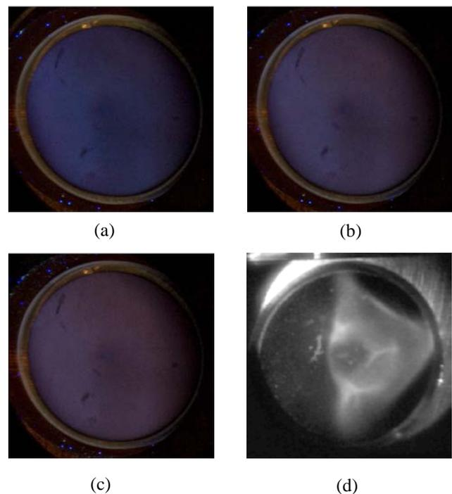
**Fig. 2.** Optical images of luminescent SiO<sub>2</sub> samples. SLR still images of the glowing thin film SiO<sub>2</sub> sample at (a) 273 K, (b) 193 K and (c) 163 K. Note that the lower temperature image has a very red tint to it. However, as the temperature continues to rise, and eventually reaches room temperature, the color begins to shift to blue. (d) CCD video camera frame showing the luminosity produced by a highly distorted, defocused electron beam.
