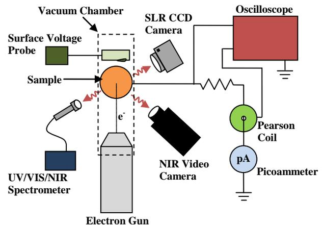
**Fig. 1.** Block diagram of instrumentation for collecting the pulse charging surface voltage, electrode current and cathodoluminescence data induced by electron beam bombardment. Instrumentation includes picoammeters, Pearson coils, and a storage oscilloscope for electrode current measurements and UV/VIS and IR spectrometers, an SLR CCD still camera, and a NIR video camera for optical measurements.
