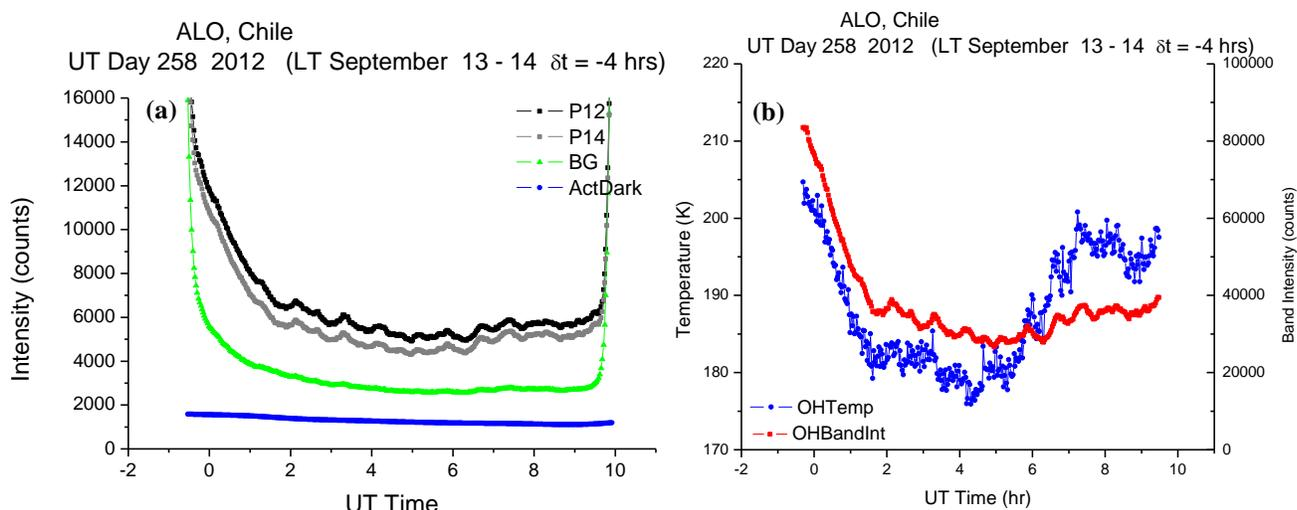
**Figure 5.** MTM temperature data for September 13-14, 2012. (a) plots the OH emissions (shown in black and grey), the background (green) and the dark (blue) intensities. (b) plots the OH band intensity (red) and the derived OH temperature (blue).
