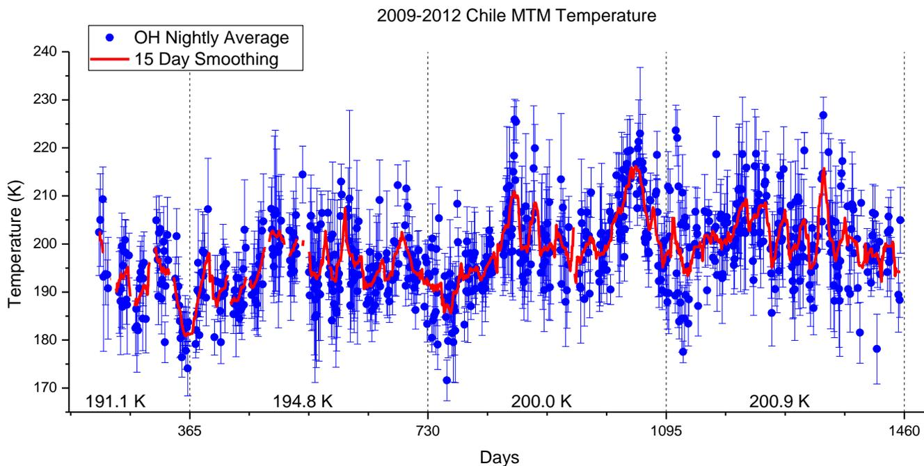
**Figure 6.** MTM nightly averaged OH temperature measurements from August 12, 2009 until December 31, 2012. Days are counted from January 1, 2009, where years are separated by black vertical lines. The blue points are the mean temperature for each night and the error bars represent the standard deviation in temperature each night. A 15 day running average smoothing fit (red line) is applied to the data.
