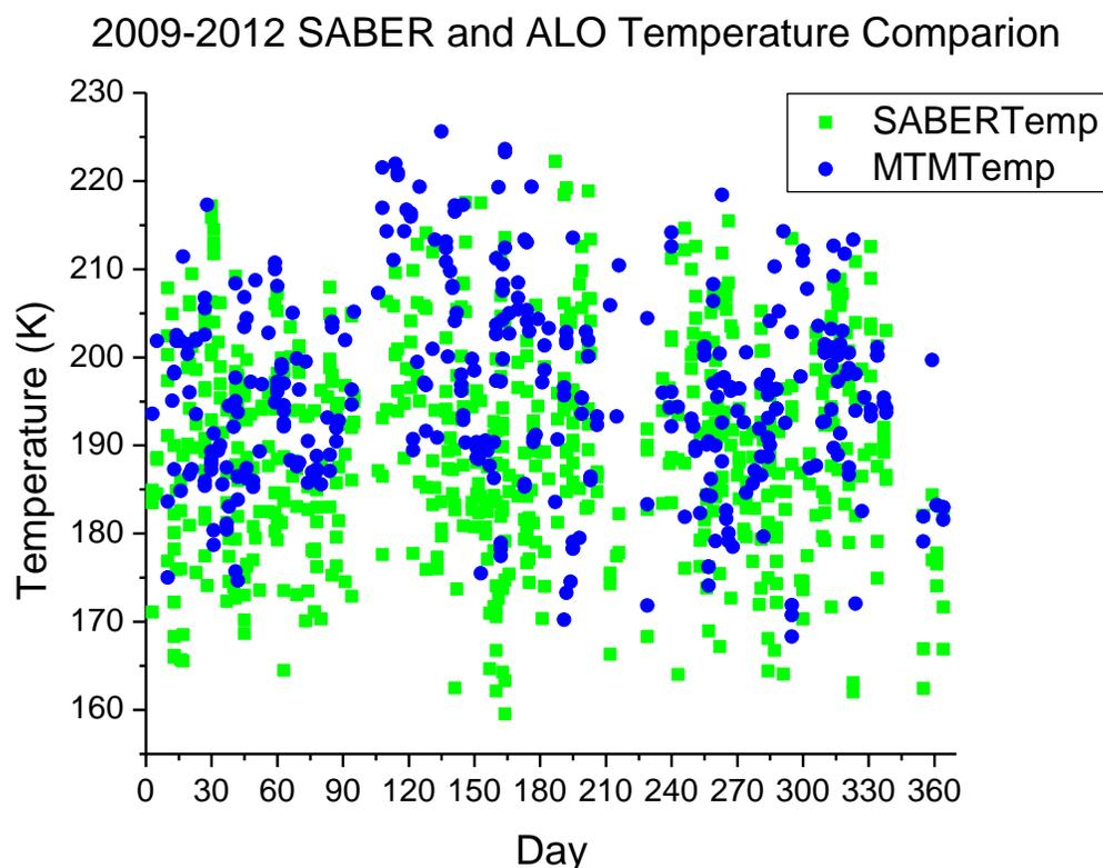
**Figure 9.** Coincident SABER temperature measurements and MTM OH temperature measurements for August 2009 to December 2012 folded into one year. SABER average temperature is 190.2 K and MTM OH average temperature is 195.9 K.
