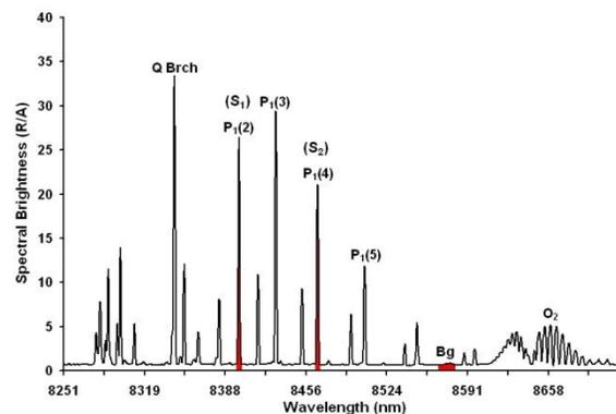
**Figure 3.** Emissions given by different OH vibrational mode transitions. The ratio of the P<sub>1</sub>(2) to P<sub>1</sub>(4) emissions (highlighted in red) is used to measure OH rotational temperature.
