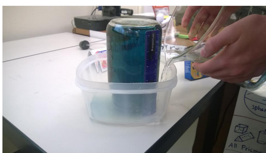
Figure 4: After inverting the jar add additional water (about 1 cm) to help maintain the seal.
