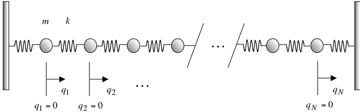
Figure 7. Linear chain of coupled oscillators. Each oscillator of mass  $m$  is coupled to its nearest neighbor with a spring with spring constant  $k$ . As in the case of the two-coupled oscillator problem, displacement from equilibrium  $q_i$  is restricted to be along the chain of oscillators, as illustrated.
