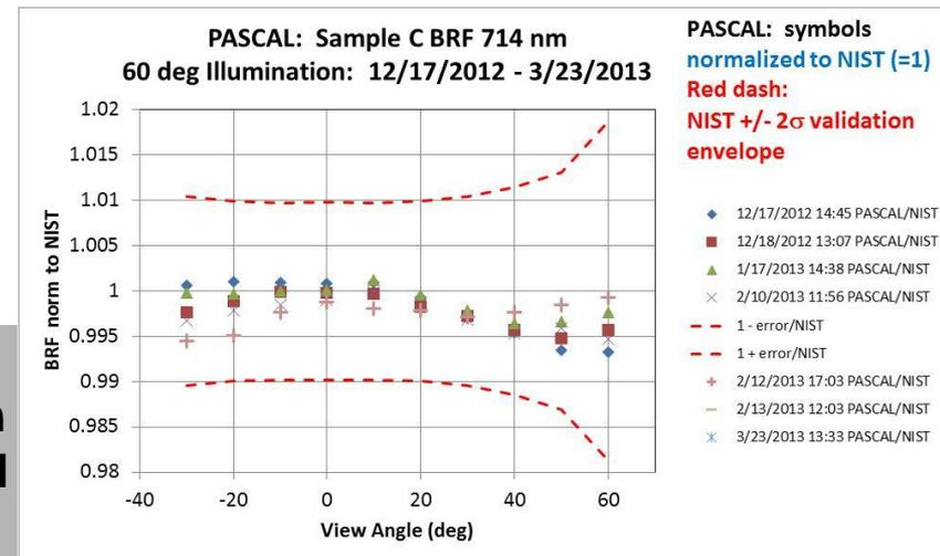
**PASCAL measurements are within NIST validation envelope for -30° to 60° viewing angles for 60° AOI**
