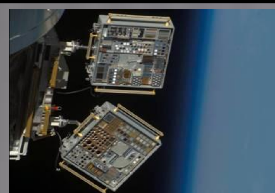
Figure 2: Space environment exposure of MISSE-6 samples in various locations
