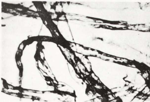
Fibrous Cellulose from Wood Pulp 375X
