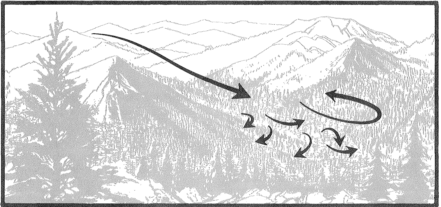
Ridgetop saddles and mountain passes form important channels for general wind flow. The flow converges and the wind speed increases in the passes. Horizontal and vertical eddies form on the lee side of saddles.
