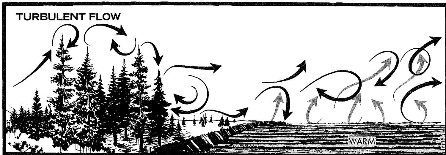
Roughness creates mechanical turbulence, while surface heating causes thermal turbulence in the airflow.
