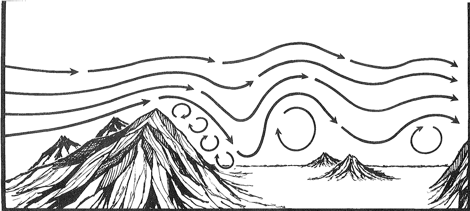
Mountain waves form when strong winds blow perpendicular to mountain ranges. Considerable turbulence and strong updrafts and downdrafts are found on the lee side. Crests of waves may be marked by lens-shaped wave clouds, but at times there may be insufficient moisture to form clouds.
