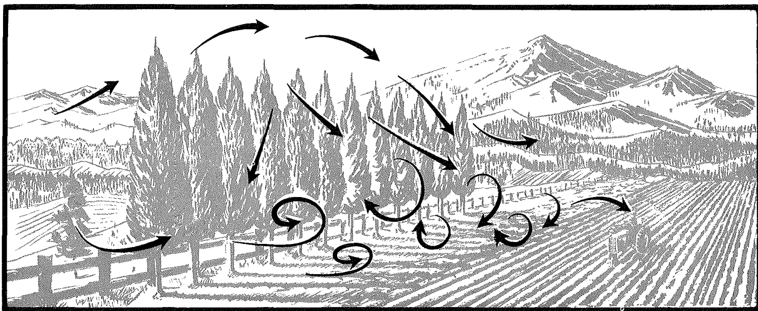
Eddies form as air flows over and around obstacles. They vary with the size and shape of the obstacle, the speed and direction of the wind, and the stability of the lower atmosphere.
