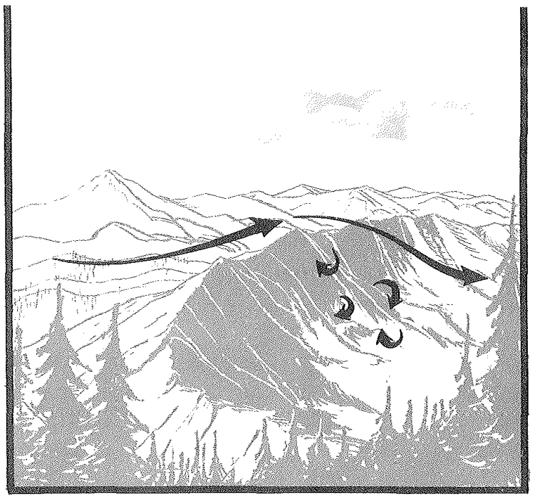
Higher wind speeds and sharp ridges cause turbulence and eddies on the lee side.
