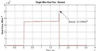
Figure 4 – Heat flux during burnout of single wire
