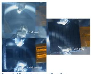
Figure 1 - Microheater array configurations
