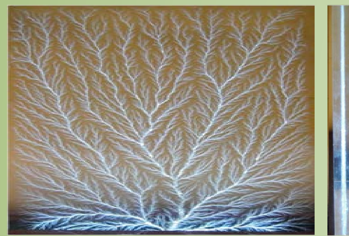
Fig. 2. Front (Left) and side (Right) views of a Lichtenberg discharge tree. The white line (Right) indicates the narrow distribution of deposited charge from a ~1 MeV electron beam at R=3 mm in a PMMA sample.
