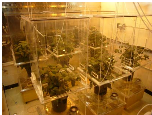
Figure 3-1. Soybean plants in growth chambers used for ethylene synthesis experiments.
