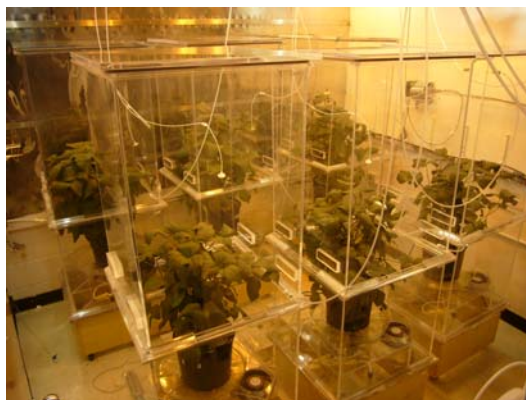
Figure 4-1. Soybean plants in growth chambers used for ethylene synthesis experiments.
