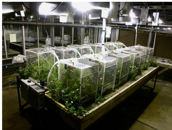
Figure 2-2. Pea plants growing in greenhouse system. Each chamber was individually controlled for temperature and ethylene mix. Lighting was controlled by screening each chamber. Each row was treated as a block in a randomized complete block experiment design. Photo has been color corrected.
