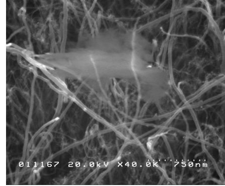
Fig. 3. Formation of a large crystal on top of CNT forest
