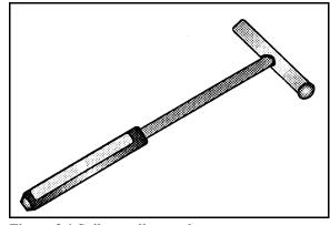
Figure 2.1 Soil sampling probe.
