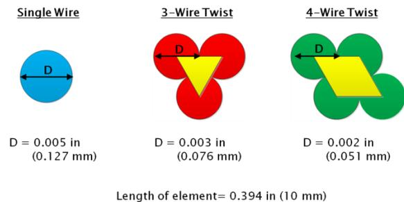
**Figure 1 – Heating Element Wire Geometries from FUNBOE**
