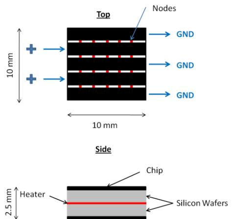
**Figure 2 – Proposed Surface Heater Design**
