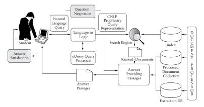
Figure 11.1. System Architecture
