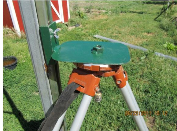
Figure 2 – Calibration stand mount on tripod
