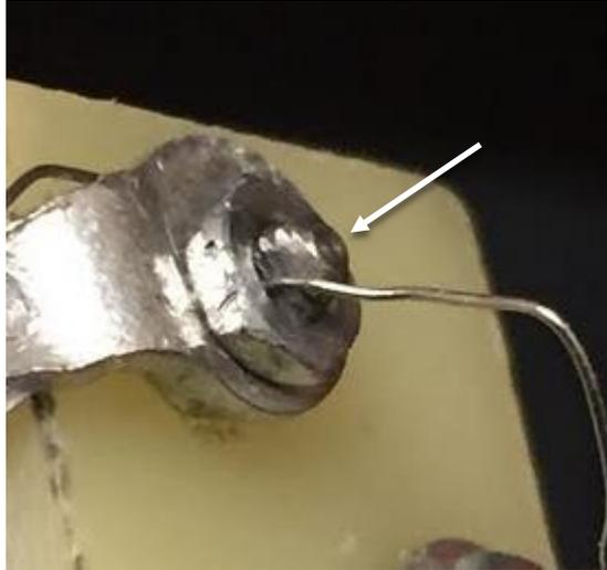
**Figure 13.** Close up of NCWC filament terminal (Note pin threads are faced in order to prevent slipping of the filament wire, it is at this interface that additional testing with thermal adhesives should be conducted)
