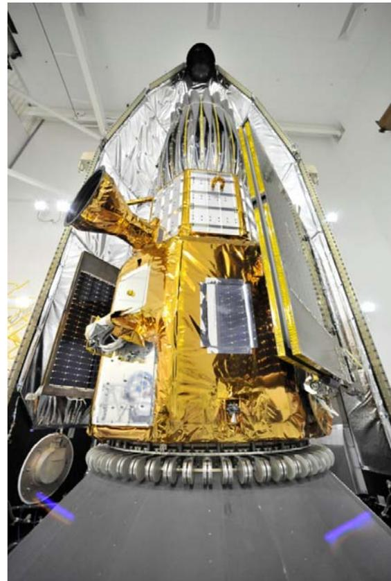
Figure 4. TacSat-4 During Fairing Encapsulation
