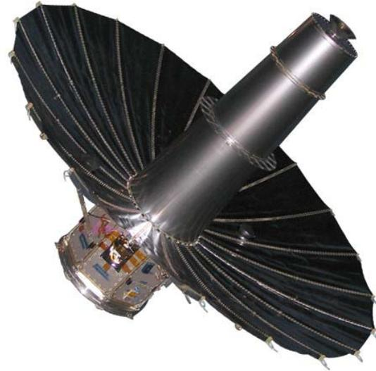
Figure 2. COMMX Payload with its Reflector Deployed
