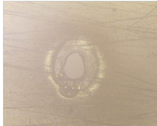
Figure 3.0. Melt ring surrounding damage
