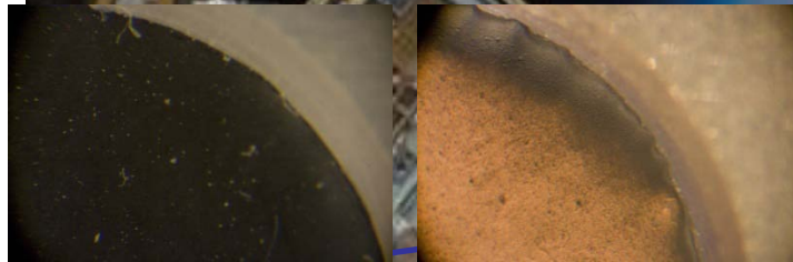
Before After Black Kapton Surface modified by AO, UV
