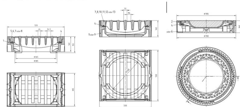
Figure 5. Exemplary gully geometries, left: 300 mm x 500 mm,  $A = 0.0515 \text{ m}^2$ , middle: 500 mm x 500 mm,  $A = 0.0815 \text{ m}^2$ , right: example of a manhole with an inlet area  $A = 0.025 \text{ m}^2$  (DIN-19583-1, DIN-19594-1, DIN-19584-1)
