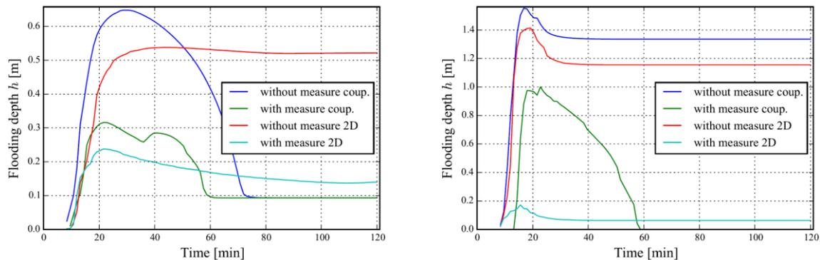
Figure 11. Exemplary results for the comparison of implemented measures at two points within the modelled catchment area for a simple 2D surface model and 1D-2D coupled model, left: a low point on the street, without and with retention basin as measure, right: a low point in front of a house without and with gully as measure,  $T = 100a$  and  $D = 10$  min
