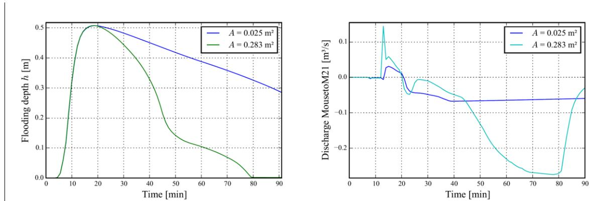
Figure 7. Comparison of manhole inlet area variation ( $A = 0.025 \text{ m}^2 =$  aerated area and  $A = 0.283 \text{ m}^2 =$  manhole fully opened), left: influence on flooding depth and flood duration, right: influence on exchange rate (discharge MOUSE to MIKE21)  $T = 100\text{a}$  and  $D = 30$  min.
