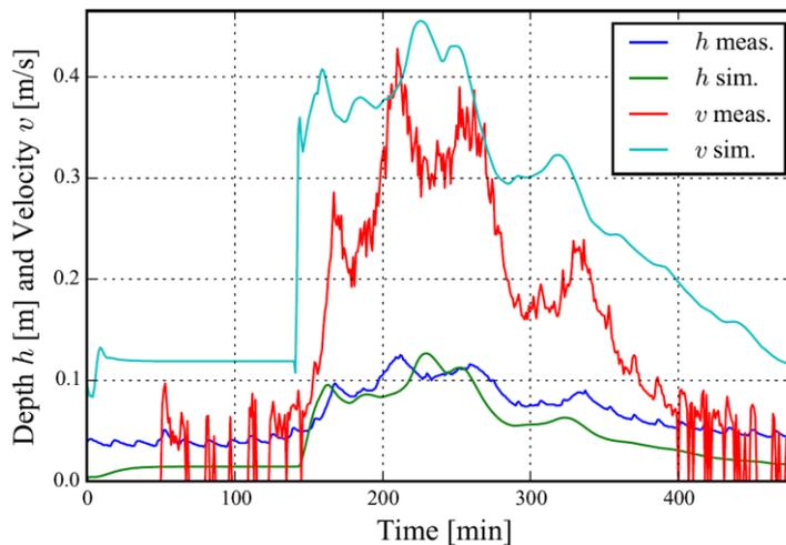
Figure 10. Comparison of measured water depth and flow velocity and simulated results for these parameters with the 1D model, duration from 8 a.m. until 4 p.m. at the 15<sup>th</sup> of April 2016
