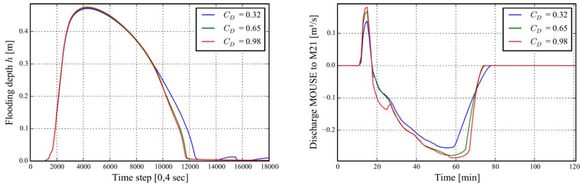
Figure 9. Comparison of discharge coefficient variation, left: influence on flooding depth and flood duration, right: influence on exchange rate (discharge MOUSE to MIKE21),  $T = 100a$  and  $D = 10$  min
