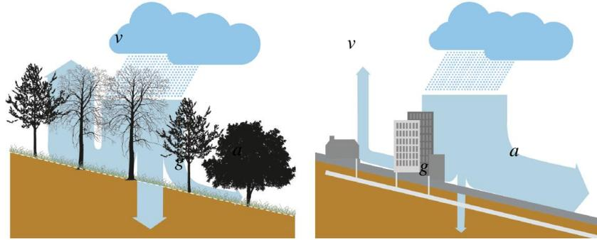
Figure 1. Increase of runoff ( $a$ ) due to surface sealing and decrease of infiltration ( $g$ ) and evapo-transpiration ( $v$ ) in urban areas (Kruse et al. 2014)
