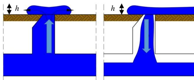
Figure 4. Schematic plot of coupled nodes (manholes and gullies) with bi-directional exchange of water between 1D-2D model, left (1): surcharge, right (2): inflow from 2D overland (DHI, 2015)
