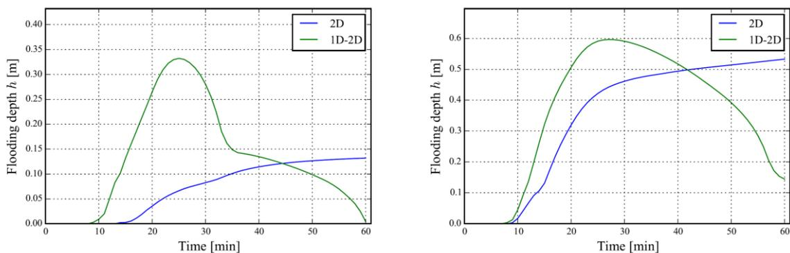
Figure 6. Comparison of exemplary model results (flooding depth) for the simple 2D surface model (2D) and the coupled sewage-surface model (1D-2D), left:  $T = 5a$ , right: (b)  $T = 100a$  of  $D = 30$  min. (according to Kühnel 2015)
