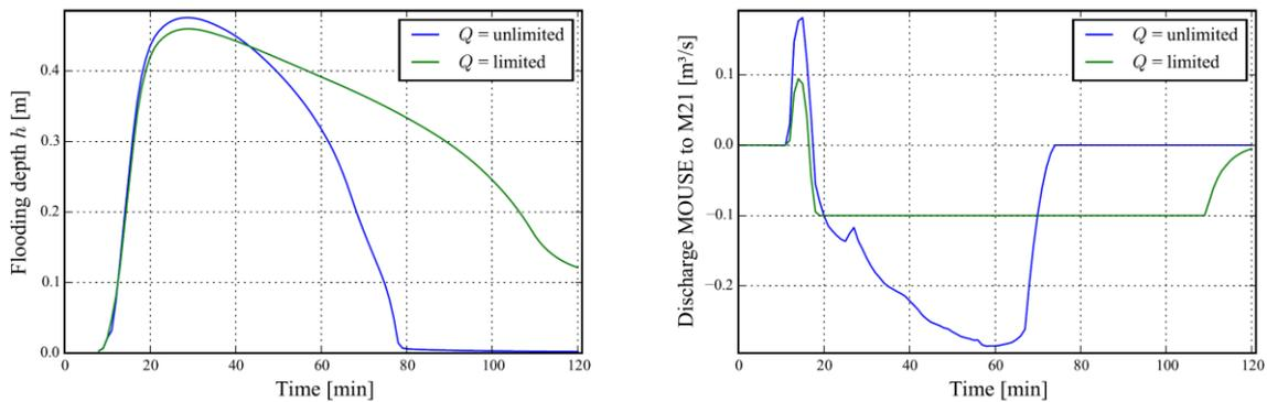
Figure 8. Comparison of limited and unlimited inlet capacity of gullies, left: influence on flooding depth and flood duration, right: influence on exchange rate (discharge MOUSE to MIKE21),  $T = 100\text{a}$  and  $D = 10$  min.
