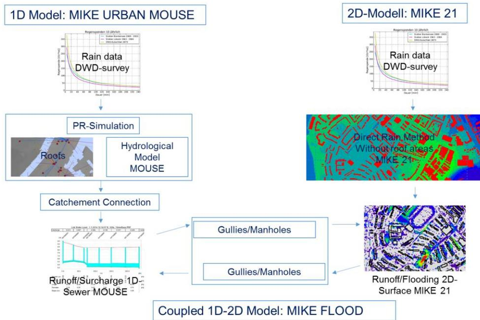
Figure 3. Schematic overview of coupling process for 1D and 2D numerical model (according to Kühnel 2015)
