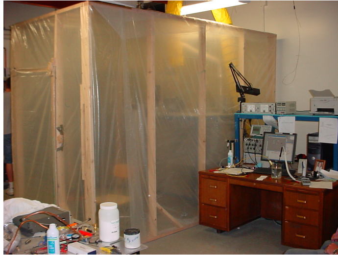
Fig. 5.6: Room built to simulate a field measurement.
