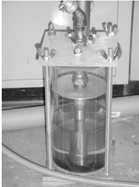
Fig. 4.4: The atomizer produces small seed particles for the PIV.
