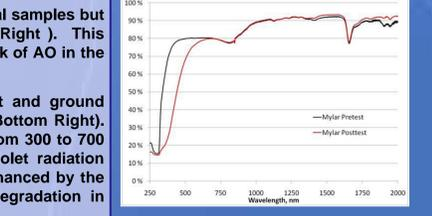
• The most noticeable change in both the flight and ground samples occurred on the aluminized Mylar (Figure-Bottom Right). Most of the loss appears within the visible region from 300 to 700 nm. This change was likely due to vacuum ultraviolet radiation severing the polymer bonds, but may have been enhanced by the electron beam as other researchers have found degradation in Mylar under energetic electron bombardment.
