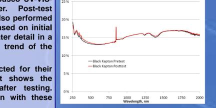
• Black Kapton had some small changes on the orbital samples but had little change in the ground test (Figure-Middle Right). This was likely due to interaction with AO on orbit and lack of AO in the ground test.
