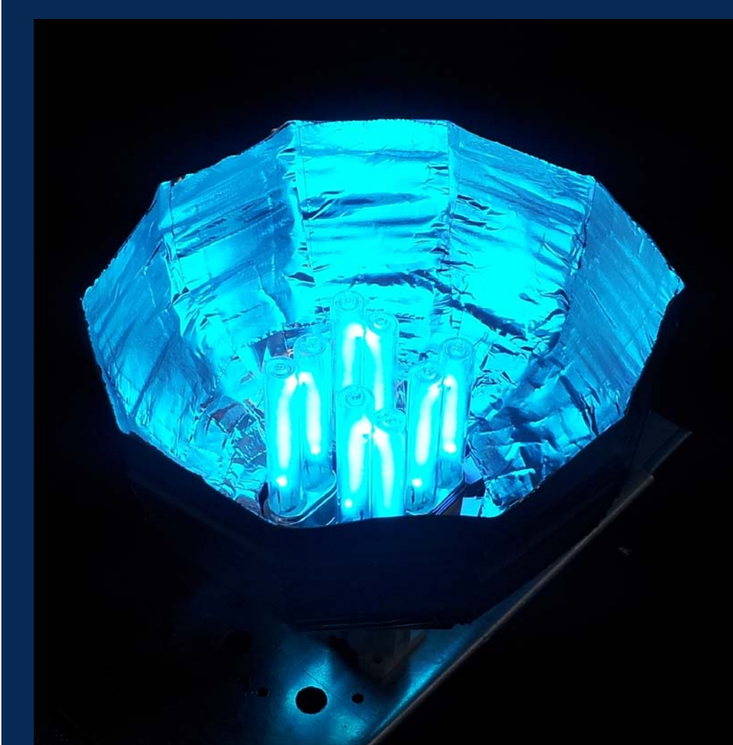
Deuterium lamp to simulate the UV solar radiation in a condensed time frame.
