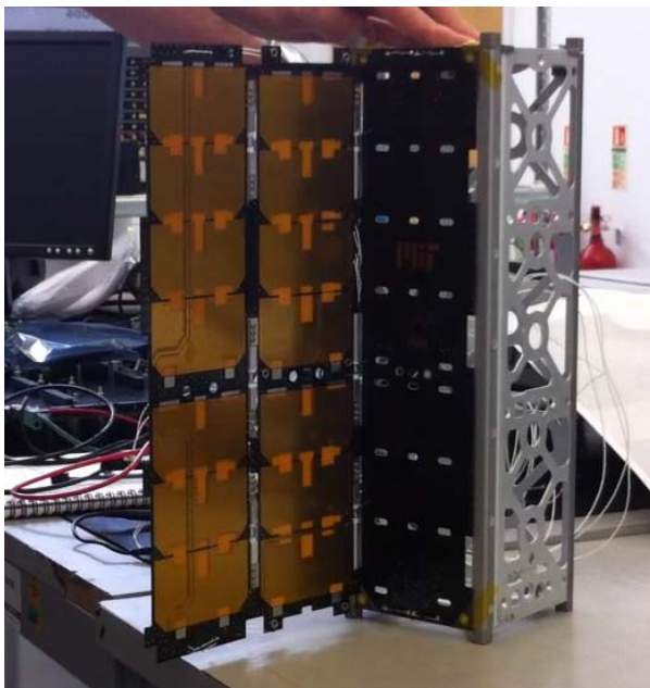
Figure 15 Deployable panels can significantly increase solar cell surface area.
