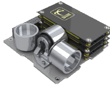
Figure 9 3D model of 3-Axis reaction wheel system incorporating a 20Whr battery.
