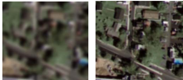
Figure 5 Comparison of the resolution of man-made structures using simulated blurring of a real EO image
