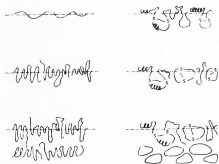
Fig. 16. Schematic representation of the structures of absorbed films of \beta -casein and lysozyme at interfaces at different surface concentration. \beta -casein (disordered, flexible) left column, lysozyme (globular, rigid) right column. Surface concentration top row << \Gamma_{sat} , middle row \approx \Gamma_{sat} , bottom row > \Gamma_{sat} . (Source: Graham and Phillips, 1974. Reproduced with permission).
