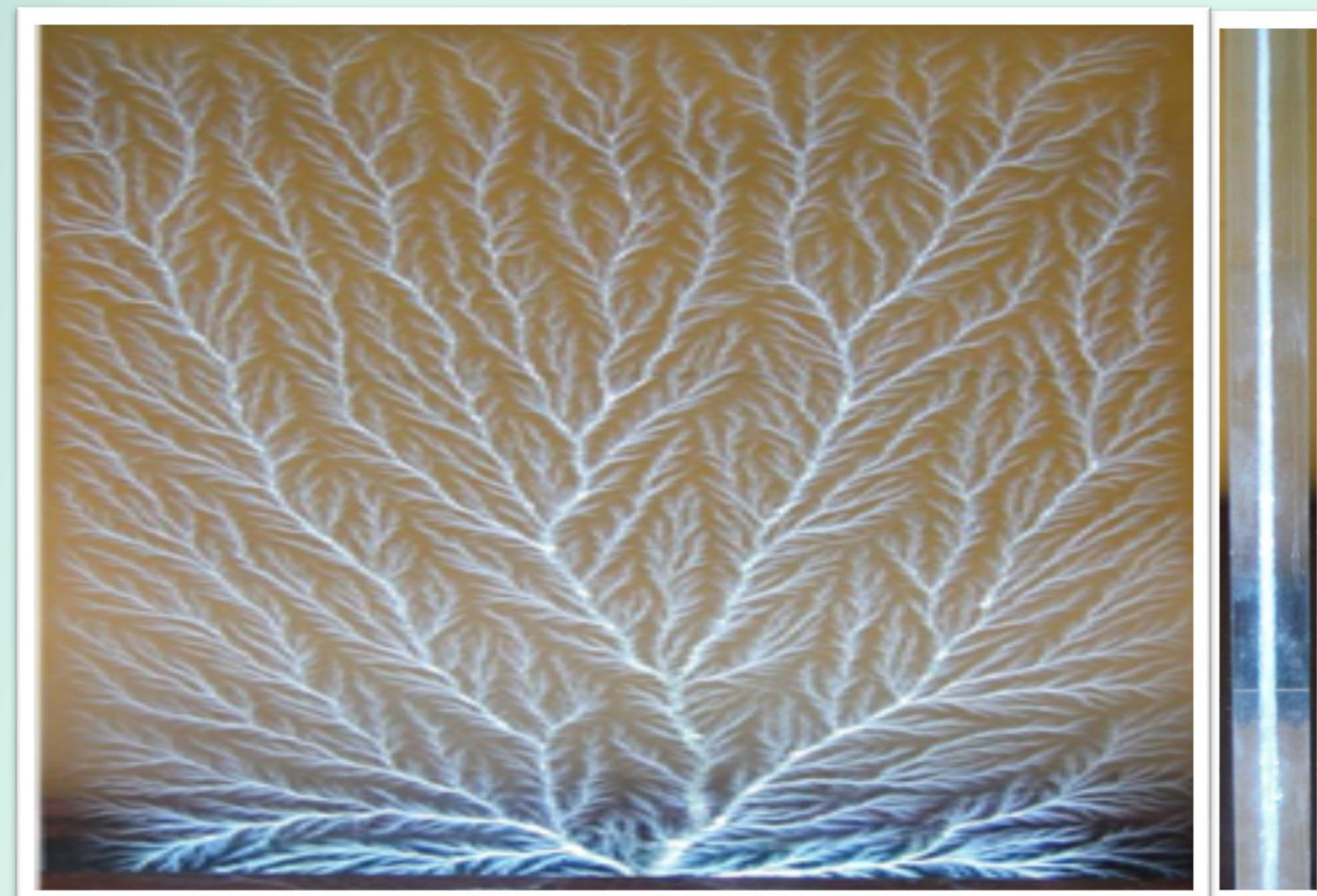
Fig. 1. Front (Left) and side (Right) views of a Lichtenburg discharge tree. The white line (Right) indicates the narrow distribution of deposited charge from a ~1 MeV electron beam at R=3 mm in a PMMA sample.
