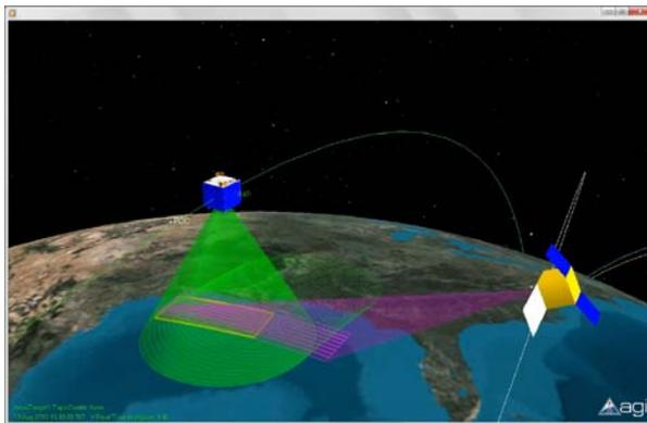
**Figure 4: SAR/AIS Coverage Simulation**
