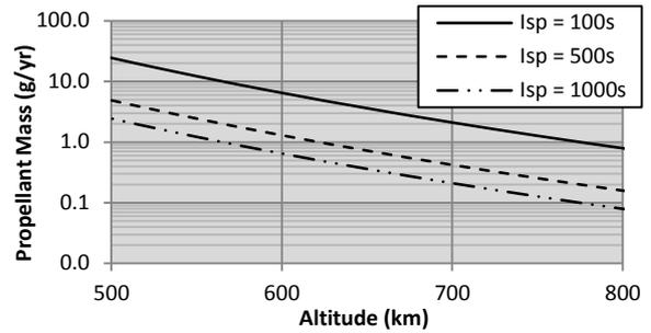
Figure 7: Plot of Propellant Mass (g/yr) required to compensate for Drag, vs. Orbit Altitude (km)
