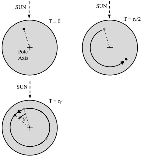
**Figure 2: Angular rotation of Earth after one TLD**
