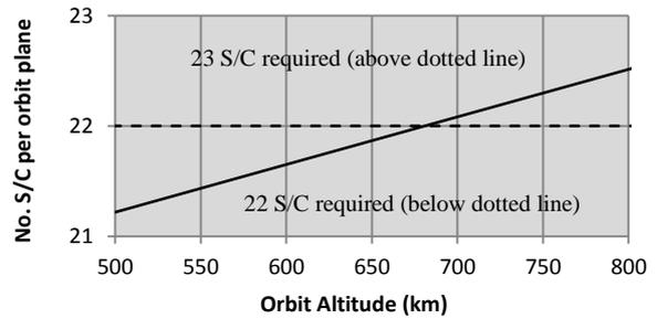
**Figure 4: Plot of  $N_{S/C}$  vs. Orbit Alt (km)**
