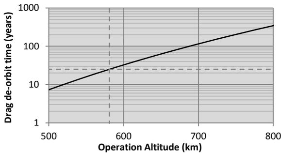
**Figure 8: Drag De-orbit time (years) vs. Operational Orbit Altitude (km)**
