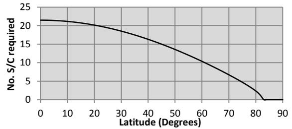
**Figure 6: No. S/C required for complete Latitude coverage vs. Latitude**
