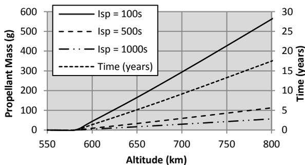
**Figure 9: Fuel required & time to decay to Critical Altitude vs. Operational Altitude**
