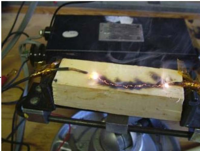
Figure 5: Conductive arc-track in wood
