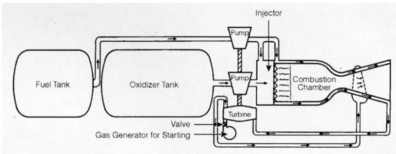
Figure 2: Basic liquid rocket design
