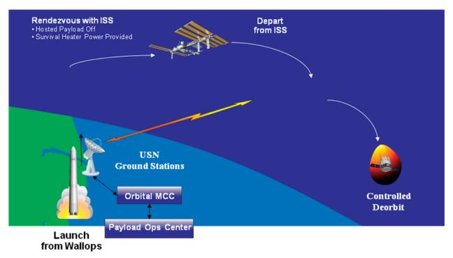
Figure 2: Notional CRS Concept of Operations
