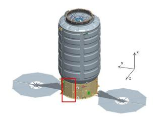
Figure 5: Potential rideshare mounting location on external service module
