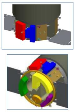
Figure 6: Example rideshare volume allocations on +Z (top) and -X (bottom) faces of Cygnus service module
