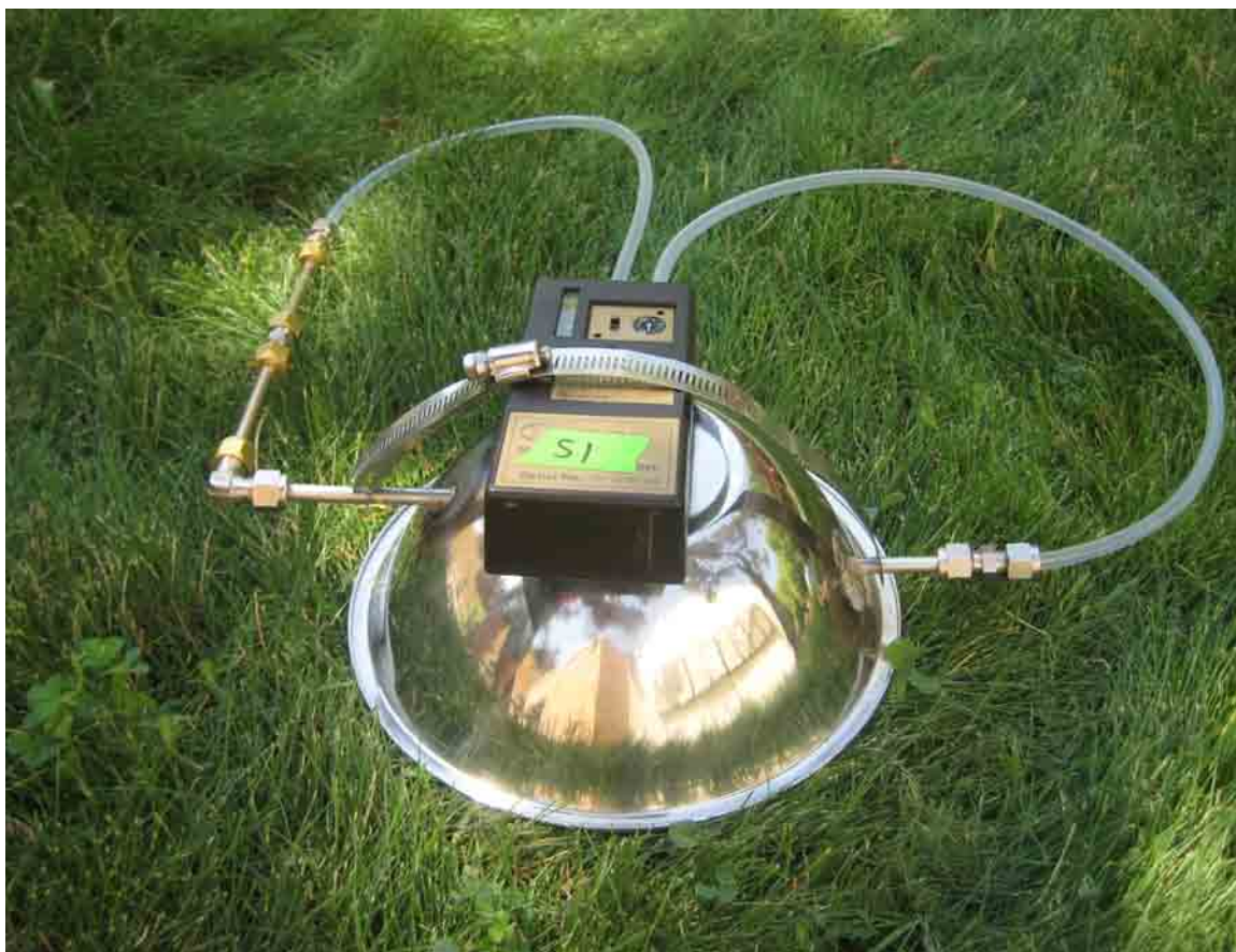
Figure 9. Soil vapor flux sampling apparatus with re-circulating pump and Tenax traps.
