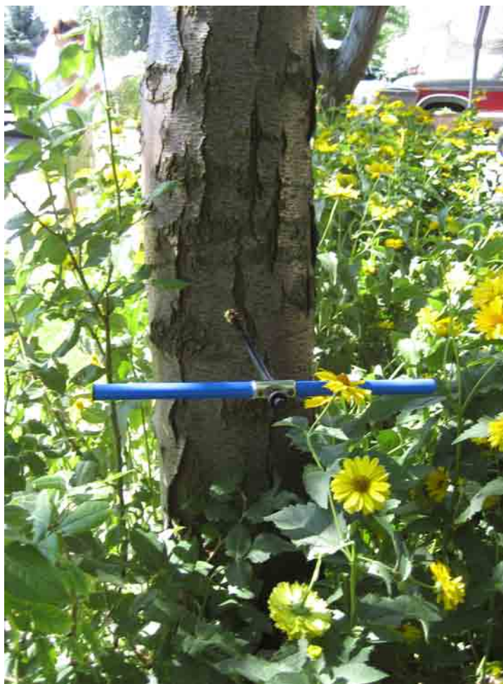
Figure 10. Incremental borer used collect tree cores.
