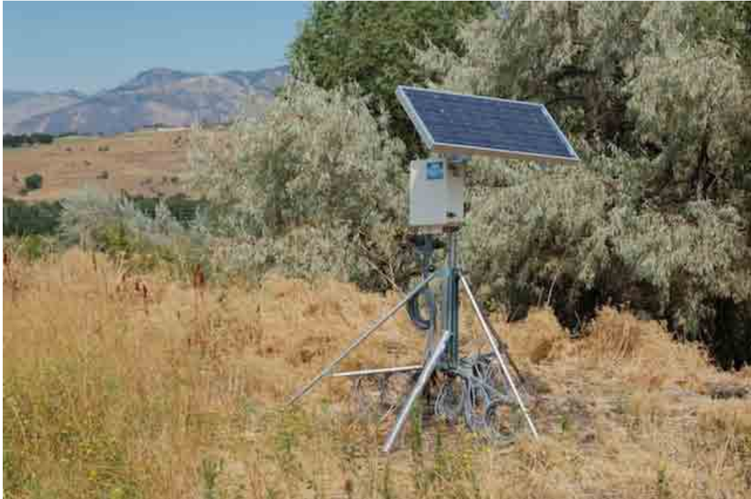
Figure 4. Datalogger and solar panel for sap flow velocity meter below OU2 canal and above sampled trees.
