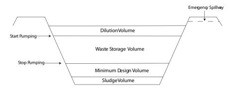
Figure 1. Single-stage anaerobic lagoon cross-section
