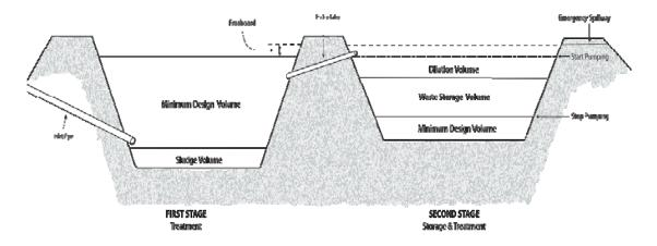
Figure 2. Two-stage anaerobic lagoon cross-section
