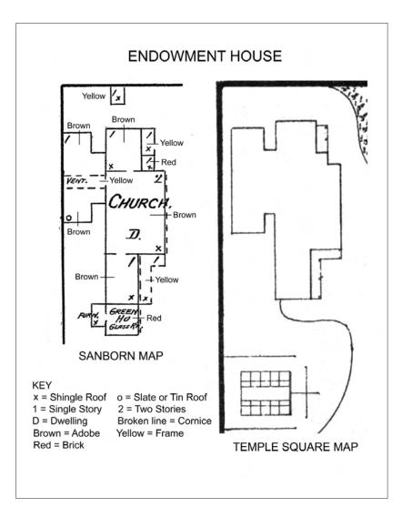
Plate 5. Diagrams of the Endowment House, enlarged from maps in House of the Lord (Cannon, 1893), 22, and Sanborn 1889 Salt Lake City Maps, sheet 10. The original Sanborn map is color-keyed; I have added the color names to the plate.
