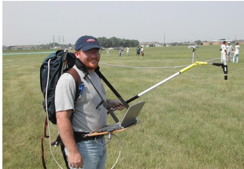
Portable spectrometer for surface reflectance measurements at a vegetated site (Image courtesy of Dennis Helder, SDSU)
