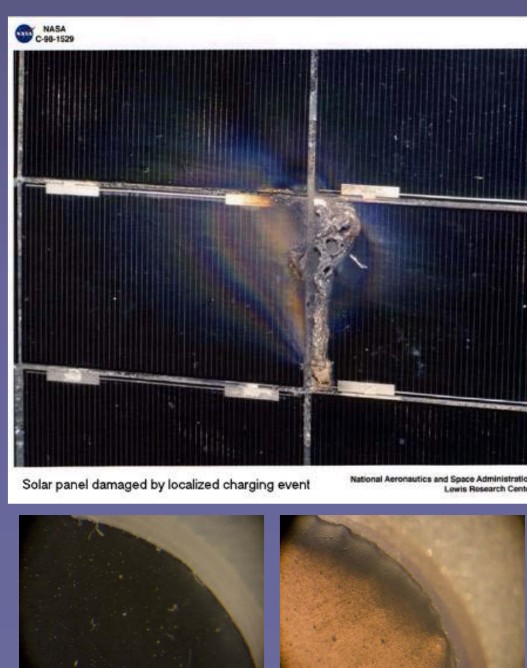
Fig. 6. (Top) Damaged Solar Panel due to overcharging. (Middle/Bottom) Photographs and UV/VIS/NIR spectra comparing pre- and post-flight samples from SUSPECS II
