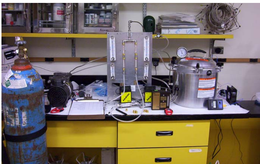
Figure 12. Photograph of the emission chamber sampling apparatus.
