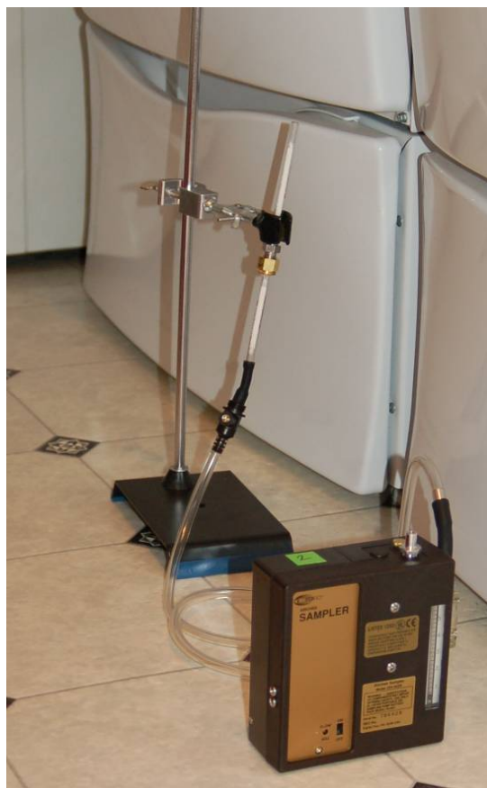
Figure 10. Area air sample apparatus setup.
