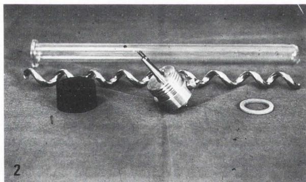
**Figure 2.** The basic components of the graft holder, i.e., the glass chamber, the steel stainless stabilizer, the O-ring seal, the security cap as well as the collector are illustrated.
