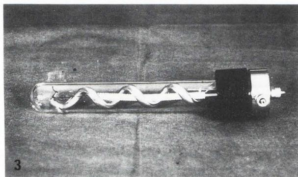
**Figure 3.** The graft holder of the rotation device with an ePTFE graft aligned on the central axis.
