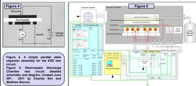
Tests were conducted in a custom, high vacuum chamber in a simple parallel plate capacitor assembly designed by the Utah State University Materials Physics Group. The concept behind the parallel plate capacitor ESD assembly can be seen in Fig. 4. However this diagram lacks the detailed setup that is required to carry out these experiments. A more detailed schematic is necessary to provide a clear analysis of any problems with the system (Fig. 5).
