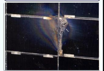
Figure 12. ESD event lead to severe damage of this solar array.
