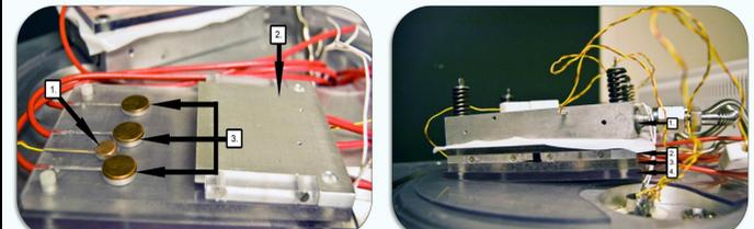
Figure 6. Exposed view of ESD sample assembly. (1) Cu thermocouple mount, (2) Sample and mounting plate, (3) Cu high voltage electrodes.
