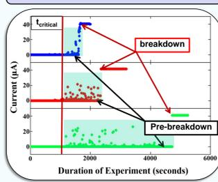
Figure 9. Three endurance curves of current as a function of time, where the applied voltage is ramped up to a set value and then allowed to sit until complete breakdown occurs. This method isolates constant applied voltage behavior from that of the ramping rate.
