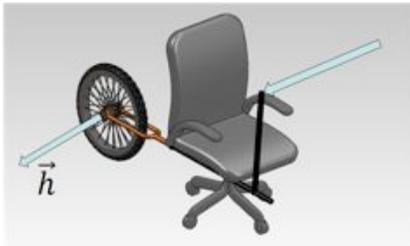
**Figure 12: When the handle indicated by the arrow to the right is pulled left, which direction does the chair rotate? Does this make sense to you?**
