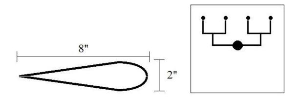
Figure 4. Airfoil - side view (left), Airfoil - internal manifold design (right)
