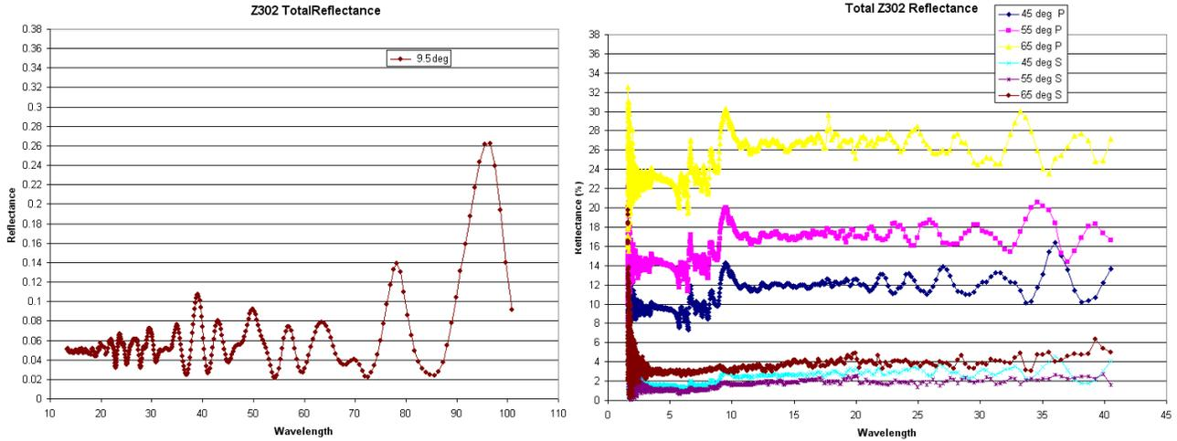
**Figure 5: Z302 total reflectance (specular and diffuse) as a function of wavelength. The plot on the left is at 8° incidence angle with polarizations averaged for 14 to 100 μm in wavelength, while the plot on the right shows both polarizations at 45°, 55° and 65° angles from 2 to 40 μm.**
