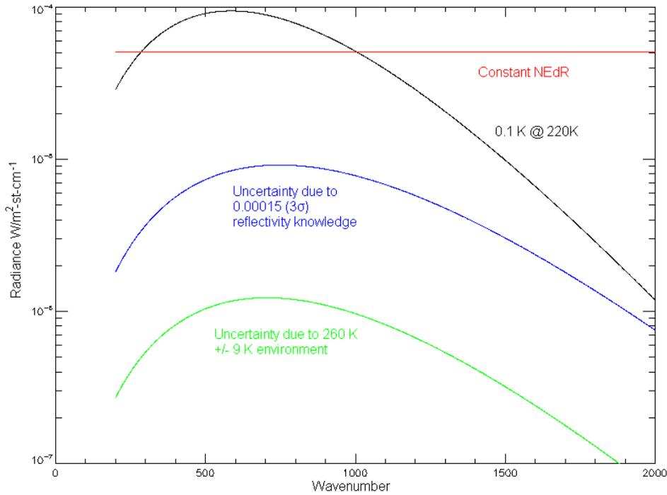
**Figure 2: The uncertainty in blackbody radiance due to uncertainty in the environment temperature and uncertainty in the blackbody reflectance for the expected CLARREO environment. The CLARREO uncertainty specifications are shown for comparison.**
