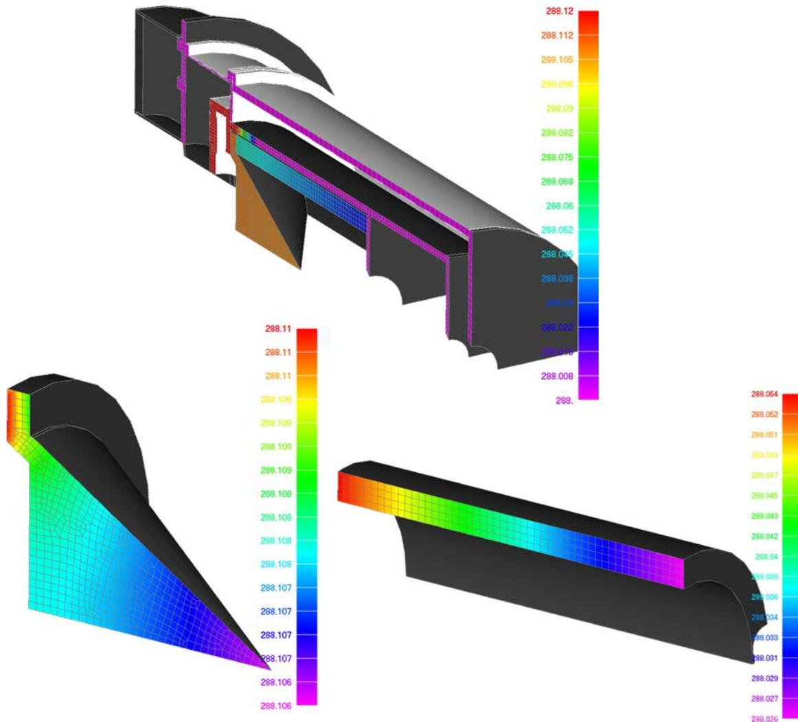
**Figure 8: Modeled blackbody gradients for a 300 K blackbody (heater set point temperature) with 77 K surroundings and the outer shield heater set point at 275 K. The top figure shows the overall blackbody, with a close-up on the cone and cylinder shown below.**
