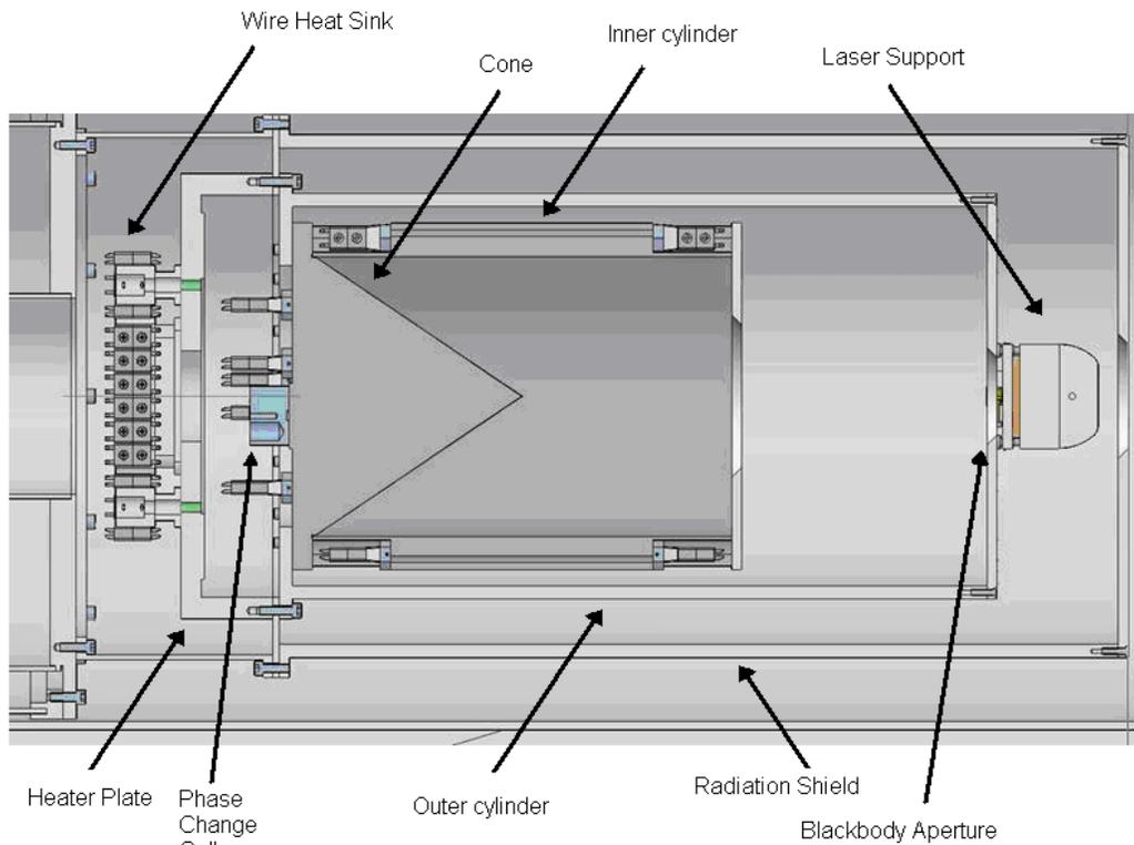
**Figure 4: A close up of the core components of the CORSAIR blackbody. The structures shown at either end of the inner cylinder and at the back of the cone are temperature sensors. The laser support is behind the aperture hole in this view and does not block the hole.**
