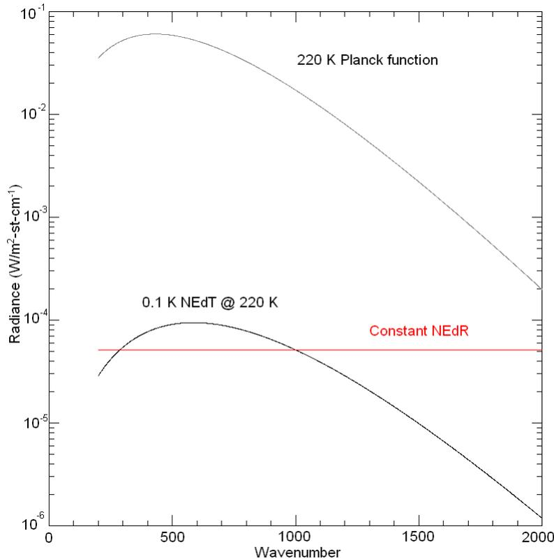
**Figure 1: The CLARREO absolute accuracy requirement SDL is using in designing the prototype blackbody, which is constant in radiance, compared to the approximate constant brightness temperature requirement and a 220 K Planck function.**
